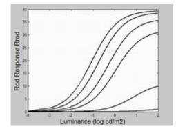
**Figure 3: Model of Rod Response.** These plots of  $R_{md}$  vs. logI were drawn with fixed adaptation intensity amounts  $I_a = 0.0005$ , 0.001, 0.01, 0.1, 1, 10 cd/m<sup>2</sup> (from left to right). Note as the adaptation intensity increases the response curve shrinks and shifts to the right. This is due to the factors  $B_{md}$  and  $F_{md}$  respectively.
