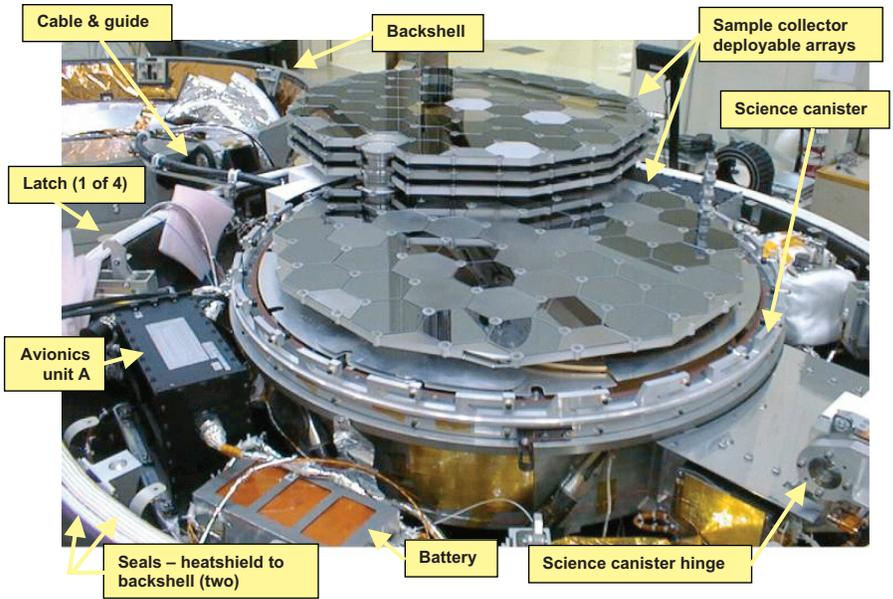
Figure 1.7. SRC prior to installing thermal closures – avionics box A and the LiSO<sub>2</sub> battery in foreground.
