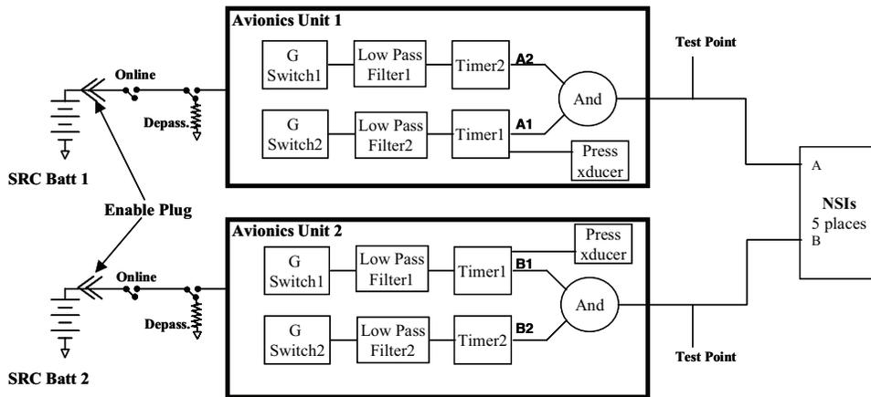
Figure 1.9. SRC pyrotechnic firing circuit layout.
