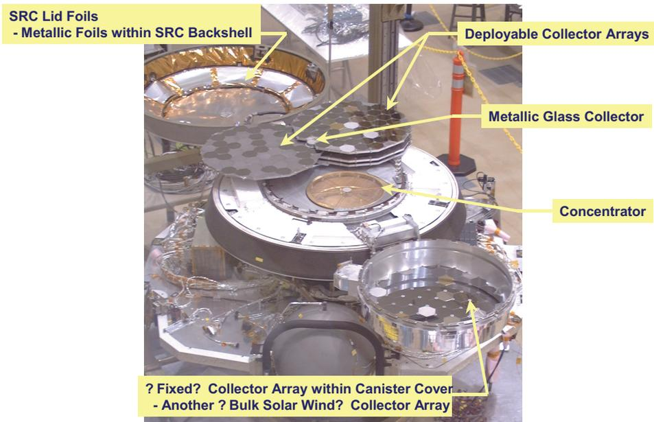
The canister is shown in the science collection configuration with the SRC backshell open and the science canister open with the arrays deployed in Figure B-5. Thermal closure panels cover the avionics and battery.
